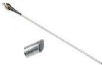
**Fiber Optic Oxygen Sensors** are made with a single 1000um fiber encased in a stainless steel ferrule or tube. The sensor end is angled. The other end is terminated with an SMA connector. These "F" style sensors are ideal for installation in compression fittings or for general lab use and are rated to withstand 55 bar. Probe length is 7" with outside diameters from 1/32" to 1/4"
